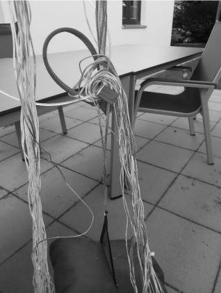
Picture 5 shows that the heavily structured release handle can cause a strong tangling / twisting with the reserve parachute 's suspension lines relatively easily and reproducibly (simulated).
