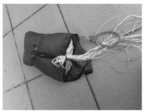
Picture 3 shows that the length of the connecting line bring the heavily structured handle into the area of the released suspension lines before the reserve parachute is released.
