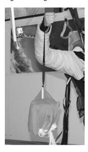
Picture 6 shows that a long connecting line from the handle to the inner container makes it difficult to throw the container because only a small arm span is available.
