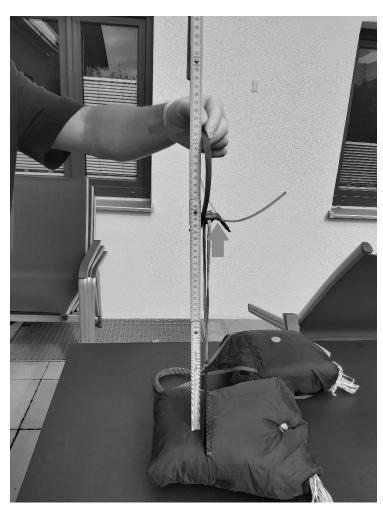
Picture 1 shows the length of the connection of 52 cm between the handle and the inner container (horizontal arrow) and the stiff strap that protrudes at right angles to the split pins (vertical arrow). In the background is an inner container of a different design with a much shorter length of less than 30 cm between handle and inner container.
